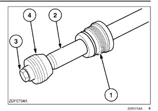
5. Slide the pre-assembled piston rod **(2)** in the cylinder housing.
