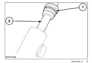
6. Tighten the cylinder head, using a punch mark and a hammer.
